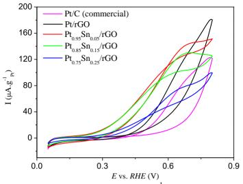
**Figure 9.** Cyclic voltammograms of N<sub>2</sub>-purged 0.5 mol·L<sup>-1</sup> H<sub>2</sub>SO<sub>4</sub>/1.0 mol·L<sup>-1</sup> C<sub>2</sub>H<sub>5</sub>OH solutions at several electrodes. The scan rate was 10 mV·s<sup>-1</sup> and all potentials were referred to the reversible hydrogen electrode (RHE) at room temperature and atmospheric pressure.
