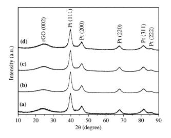
Figure 6. X-ray diffraction patterns of electrocatalysts supported on reduced graphene oxide: Pt (a),  $Pt_{0.95}Sn_{0.05}$  (b),  $Pt_{0.85}Sn_{0.15}$  (c) and  $Pt_{0.75}Sn_{0.25}$  (d).
