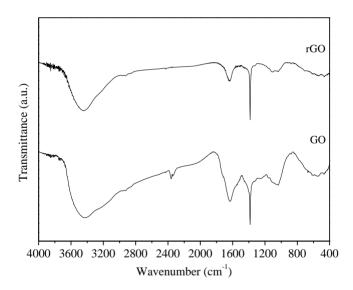
**Figure 2.** Normalized DRIFTS spectra of the synthesized graphene oxide (GO) and reduced graphene oxide (rGO).
