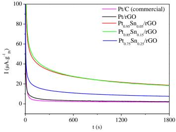
**Figure 10.** Chronoamperometric curves of ethanol oxidation at several electrodes in N<sub>2</sub>-purged 0.5  $\text{mol}\cdot\text{L}^{-1}$  H<sub>2</sub>SO<sub>4</sub>/1.0  $\text{mol}\cdot\text{L}^{-1}$  C<sub>2</sub>H<sub>5</sub>OH solutions. All measurements were carried out under a constant applied potential of 0.5 V at room temperature and atmospheric pressure.
