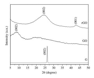
**Figure 1.** Normalized X-ray diffraction patterns of the starting graphite (G), synthesized graphene oxide (GO) and reduced graphene oxide (rGO).
