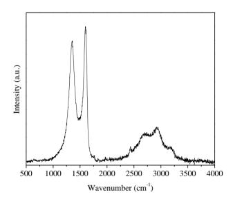
**Figure 3.** Normalized Raman spectrum of reduced graphene oxide (rGO) recorded using a 532 nm excitation laser with 1% of total power.
