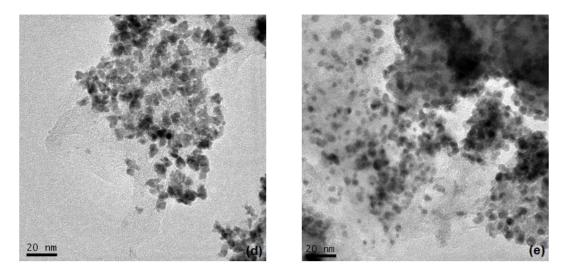
**Figure 4.** Transmission electron microscopy (TEM) images of reduced graphene oxide (a), and metals supported on reduced graphene oxide: Pt (b), Pt<sub>0.95</sub>Sn<sub>0.05</sub> (c), Pt<sub>0.85</sub>Sn<sub>0.15</sub> (d), Pt<sub>0.75</sub>Sn<sub>0.25</sub> (e).
