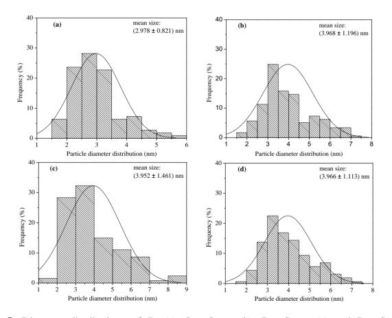
Figure 5. Diameter distributions of Pt (a),  $Pt_{0.95}Sn_{0.05}$  (b),  $Pt_{0.85}Sn_{0.15}$  (c) and  $Pt_{0.75}Sn_{0.25}$  (d) nanoparticles dispersed on the surface of reduced graphene oxide.
