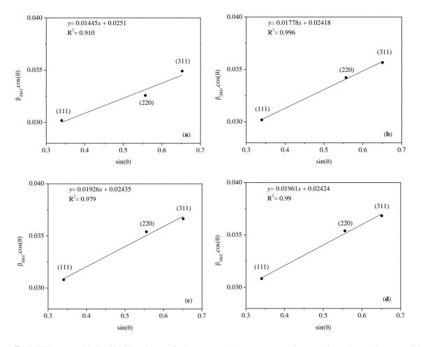
**Figure 7.** Williamson-Hall (W-H) plots of electrocatalysts supported on reduced graphene oxide: Pt (a),  $Pt_{0.95}Sn_{0.05}$  (b),  $Pt_{0.85}Sn_{0.15}$  (c) and  $Pt_{0.75}Sn_{0.25}$  (d). Each data point on the plots was labeled according to the index of its (hkl) reflections.
