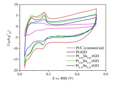
**Figure 8.** Cyclic voltammograms of N<sub>2</sub>-saturated 0.5 mol·L<sup>-1</sup> H<sub>2</sub>SO<sub>4</sub> solutions of studied electrocatalysts. The scan rate was 10 mV·s<sup>-1</sup> and all potentials were referred to the reversible hydrogen electrode (RHE) at room temperature and atmospheric pressure.
