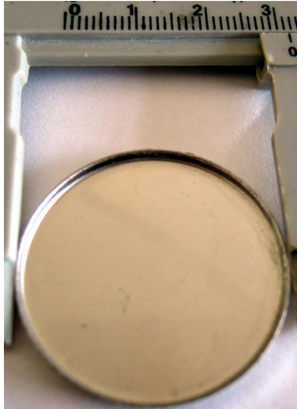
Figure 1. A view of the stainless-steel sample holder used in the measurements. Scale of the caliper rule in centimeters.
