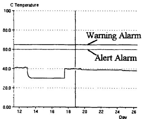
**Fig. 4: Temperature Reading from the Thermocouple at the Flywheel Bearing, Pump Side, Primary Circuit**
