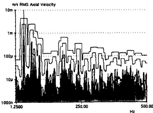
**Fig. 2: Axial Velocity Reading from the Accelerometer at the Electric Motor (Front) Bearing, Primary Circuit**
