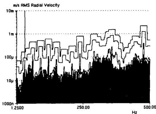
**Fig. 6: Radial Velocity Reading from the Accelerometer at the Pump (Rear) Bearing, Primary Circuit**
