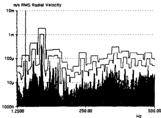
**Fig. 5: Radial Velocity Reading from the Accelerometer at the Flywheel Bearing, Pump Side, Primary Circuit**
