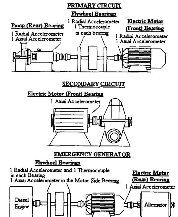
**Fig. 1: Diagram with the Transducer Positions in the Cooling Circuits and the Emergency Generator System**
