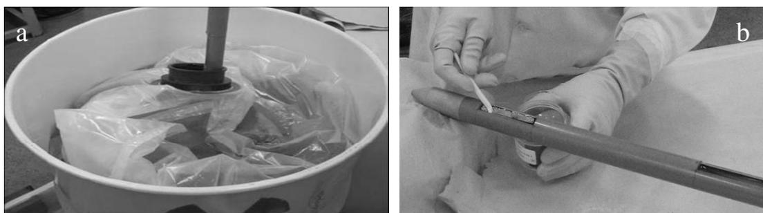
Figure 1 – Sampling of ion exchange resins: (a) thief sampler being inserted in the plastic bag that contains the waste; and (b) sample in the lower sampling port being transferred to a sample container.
