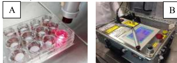
Fig.1. A – application of The CLS on 3D human skin model. B – CLS equipment.
