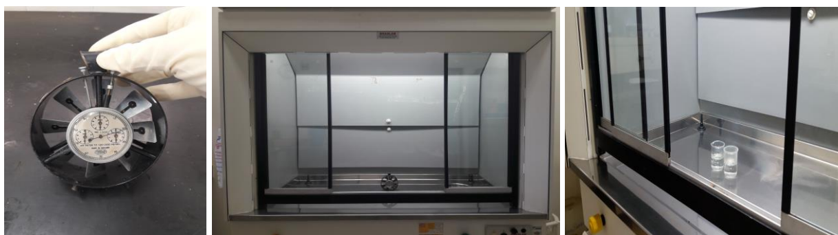
Figure 1: Left: Anemometer used in the face velocity test. Center: face velocity test with full opening windows. Right: smoke visualization test.
