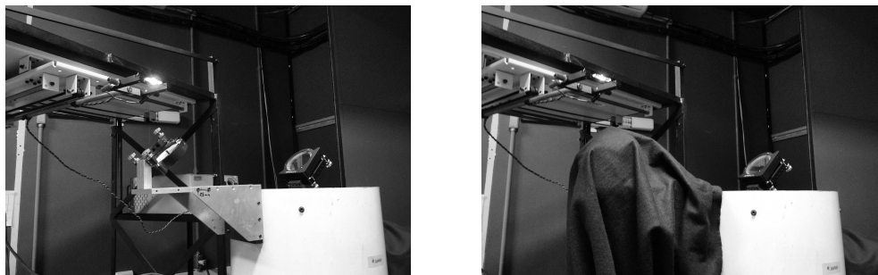
Figure 3. System configuration for different days. On the left, for the day 01/16/2014, it can be seen the the metal structure which caused the stray light. On the right, the same metal structure was covered with a black cloth in order to solve the problem.
