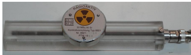
Fig. 2. Ionization chamber inside the positioning device during the stability tests
