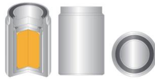
Figure 1: Typical structure of a high-activity SRS
