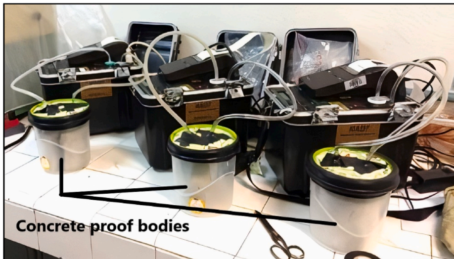
Fig. 4. Experimental apparatus for radon exhalation rate measurement in proof bodies samples.
