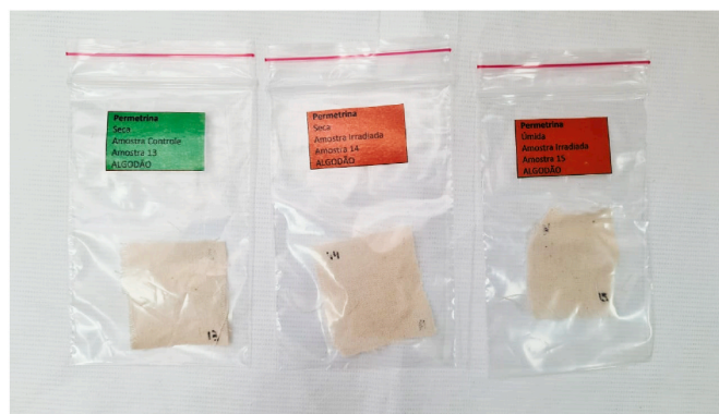
Fig. 2. Batch of cotton mock-ups contaminated with 10 ppm permethrin, separated into the three experimental conditions (control, dry and moistened).
