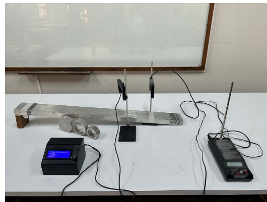
Figure 12. Experimental apparatus used in experiment (c) conservation of mechanical energy. The measurements were not carried out at the same time, due to the experimental impossibility of positioning both sensors at the same point.
