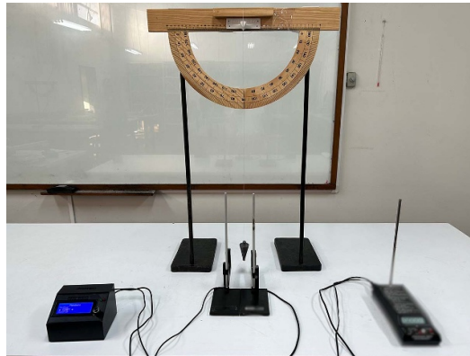
Figure 10. Experimental apparatus used in experiment (a) pendular movement. Sensors positioned side by side recording periods oscillation. From left to right: Cronpes and commercial.
