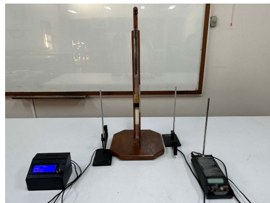
Figure 11. Experimental apparatus used in Experiment (b) spring mass oscillation. In this case, the measurements were not carried out at the same time.
