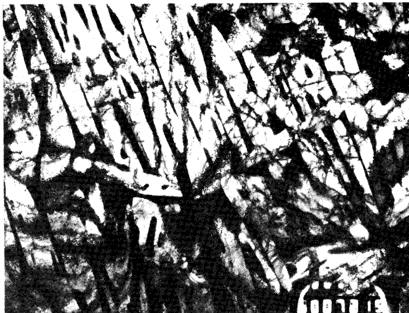
FIGURE 8. Transmission electron micrograph of Zr-2.5wt%Nb alloy tempered at 600°C for 100 hours (9000X).
