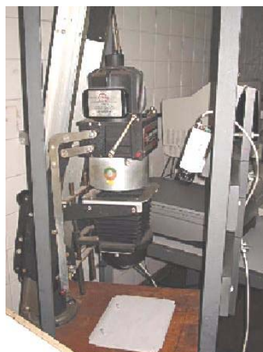
Fig 4. Digital system for light transmission analysis.
