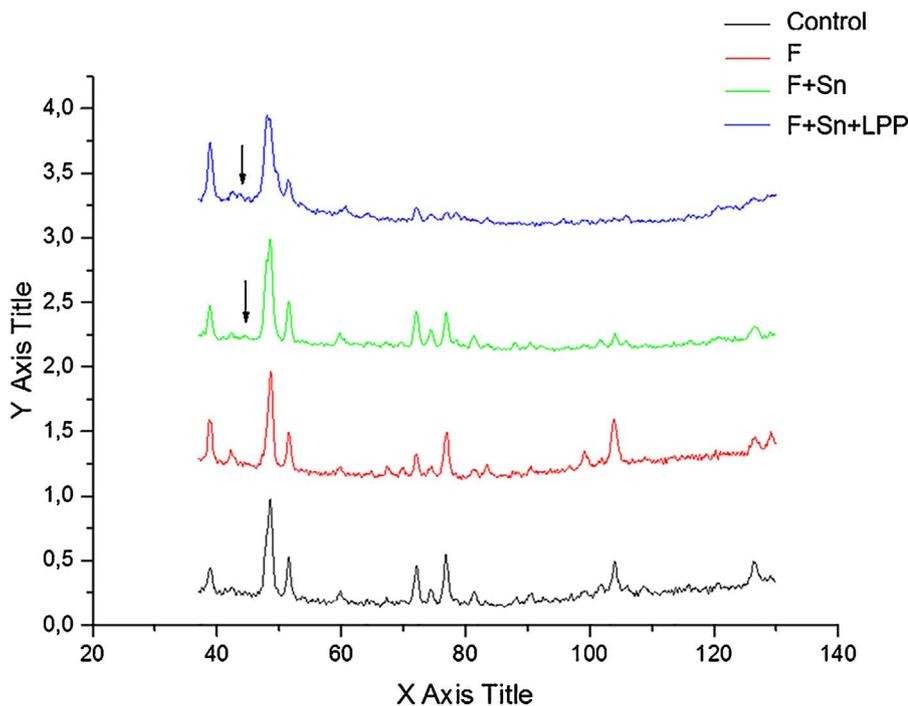
Fig. 3. Diffraction Patterns of the experimental groups, indicating the presence of apatite. The arrows suggest the presence of the phase  $Sn_3F_3PO_4$  in groups F + Sn and F + Sn + LPP.
