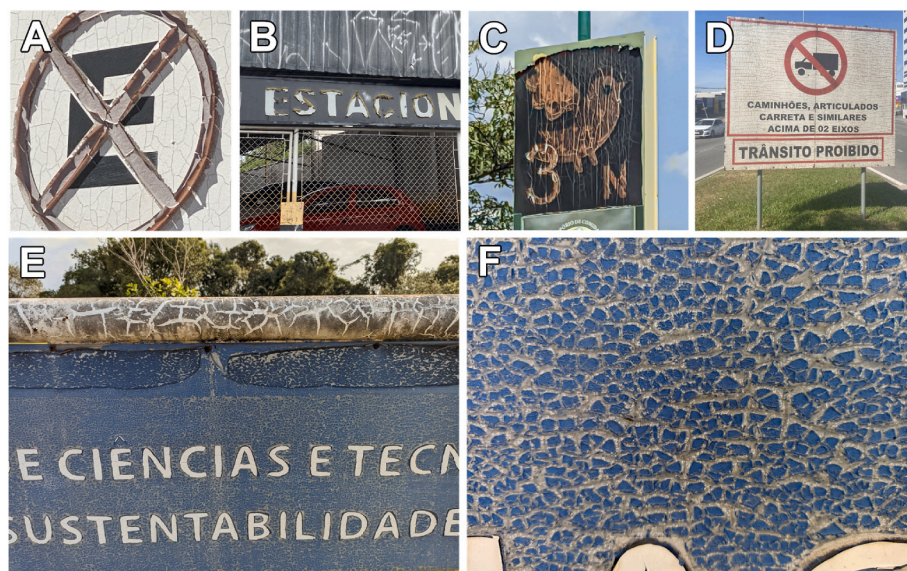
Fig. 1. Examples of everyday objects with visually degraded parts made of adhesive vinyl films: (A) No parking sign; (B) Parking banner; (C) Parking identification sign in a mall; (D) Traffic sign; (E) Sign made of adhesive vinyl that generated the MPs in the soil targeted in this study; (F) Magnification of E.
