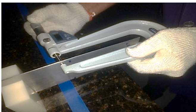
Fig. 3. Measurement of fuel plate thickness at IPEN-CNEN/SP.
