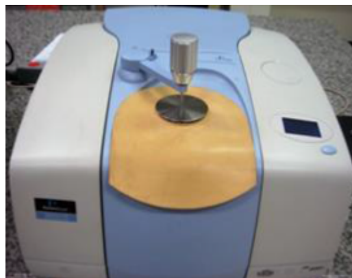
Figure 7: Fourier transformed by infrared spectroscopy analysis by spectrometer at CTR.
