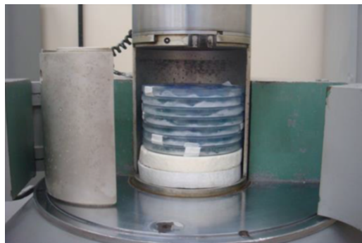
Figure 6: Placement of Petri's s plaques with different samples before submission to gamma irradiation.
