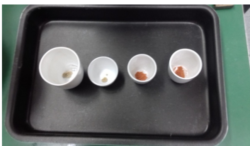
Figure 11. Ashes obtained from samples of WP (the first two on the left) and SCB (the last two on the right) after incineration in a muffle at 600 °C for 2 h.
