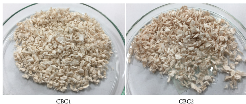
Figure 3. CBC1 (with KOH-treated residue) and CBC2 (without KOH-treated residue) cut into small pieces prior to their hydrolysis. CBC = sugarcane bagasse cellulose.
