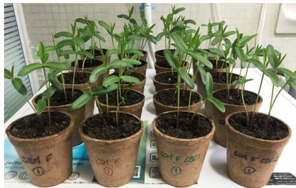
Figure 36. Crotalaria development and integrity of the different recipients in tests, after seven days of sowing. RECIPIENTS: SEM F = without film; F = film without NPCs; F-CBC1 = film with CBC1 NPCs; F-CBC2 = film with CBC2 NPCs.
