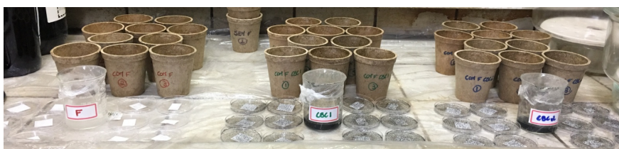
Figure 8. Recipients internally coated by a thin layer of the different film-forming suspensions (gels) and the different films formed inside the Petri dishes, after drying in the oven. RECIPIENTS/FILMS: F = film without NPCs; F-CBC1 = film with CBC1 NPCs; F-CBC2 = film with CBC2 NPCs. Additional note: the recipients were molded at Bio & Green Produtos Biodegradáveis Ltda., ex-company linked to IPEN projects.
