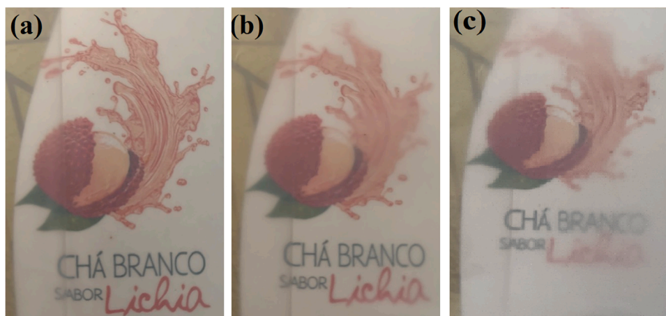
Fig. 7. Visual appearance of bionanocomposite films: (a) PBAT/PLA Blend, (b) PBAT/PLA/CNC1, and (c) PBAT/PLA/CNC2.
