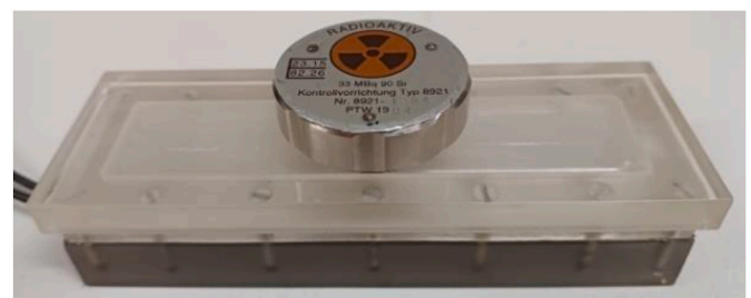
Fig. 2. Ionization chamber with a special PMMA hold and a radioactive stability checking device during stability test.
