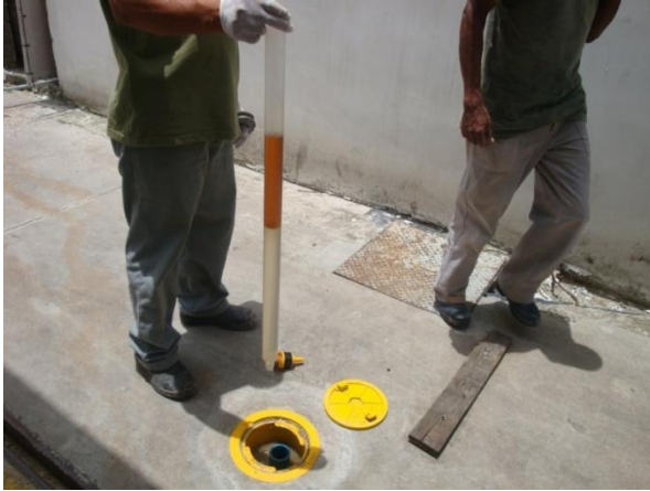
Bailer with water and LNAPL (ConAm, 2013)
