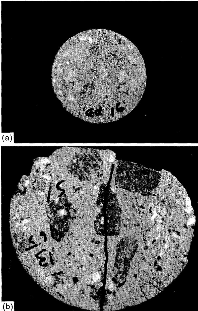
Fig. 1. (a) Conventional photograph of the S1 sample (5 cm dia) sawn from specimen type-1. (b) Conventional photograph of the S2 sample (10 cm dia) sawn from specimen type-2 submitted to compressive strength (11 MPa). Right of the divisory line with contrast agent; left without.
