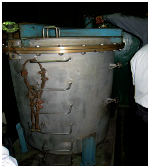
FIG. 8.13. Irradiation tank used for gamma irradiation of chitosan aqueous solution for the production of oligochitosan, 1000 m 3 per batch, in Indonesia.
