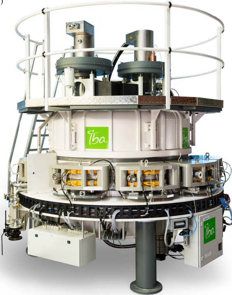
FIG. 3.1. (Cont.) The IBA Rhodotron is an electron beam accelerator able to generate beam energies of up to 10 MeV and a beam power of up to 560 kW. (a) The Rhodotron's operating principle: The electron source generates electrons which are accelerated multiple times through the cavity; when the desired energy is reached, the beam of electrons is extracted from the cavity. (b) External view. (Images courtesy of IBA.)
