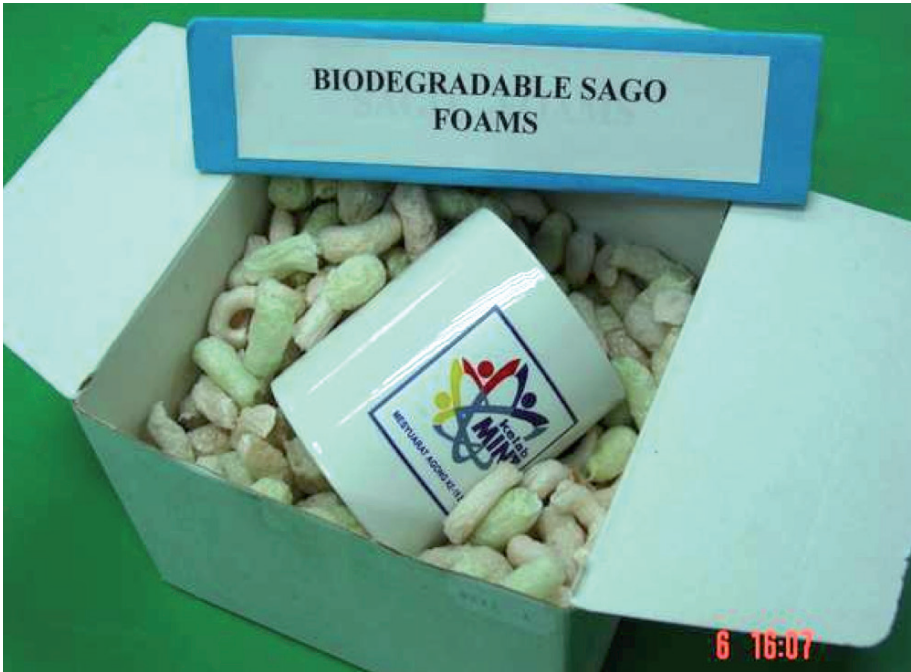
FIG. 14.4. Sago based biodegradable foam produced by radiation cross-linking of sago starch and PVA blends (photograph courtesy of Nuclear Malaysia).
