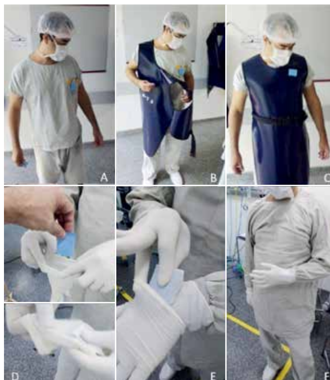
Figure 1. Attachment of film badge dosimeters to staff member body: A: lapel; B: lapel under lead apron; C: lapel over lead apron; D: inside the surgical glove; E: under sterile surgical glove; F: position on the wrist.
