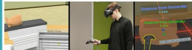
Figure 1: Educator in LINACVR (using HTC Vive). Controllers being used to view the gantry, and interacting to move the couch and position the patient model.
