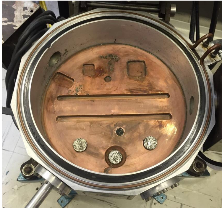
Figure 3: Samples placed in the oven, from left to right: material as received; washed with magnetic separation and washed without magnetic separation.
