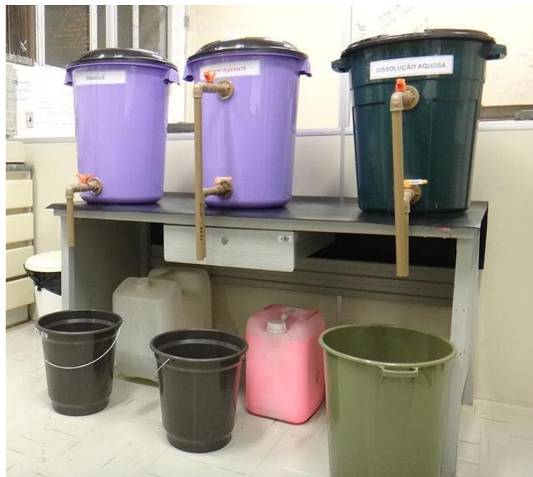
Figure 2: Cleaning station for washing of zirconium alloy chips.
