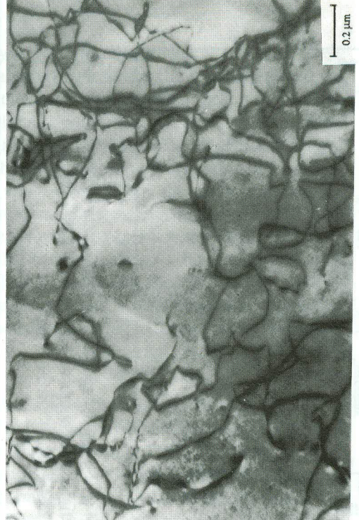
Fig. 6 Dislocation structure for the as received material 28% series B [001].
