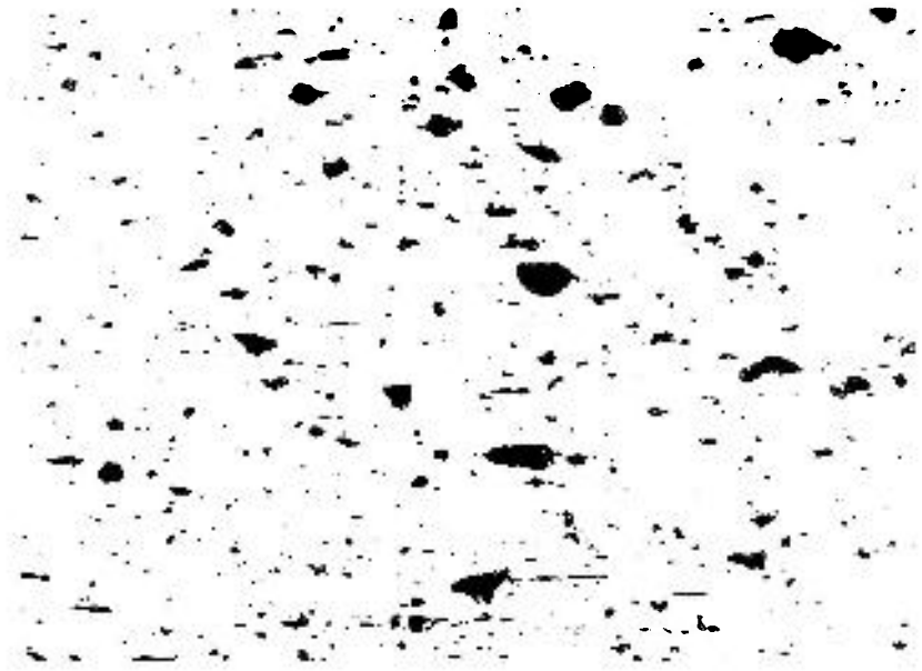
FIG. 2. Microstructure of 25% \text{UO}_2 - 75% Al core after 1000 thermal cycles; transverse section \times 80 .
