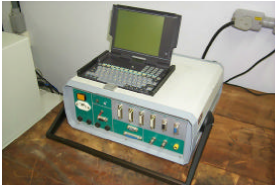
Figure 1. Magnetic Barkhausen Noise Analysis Equipment.
