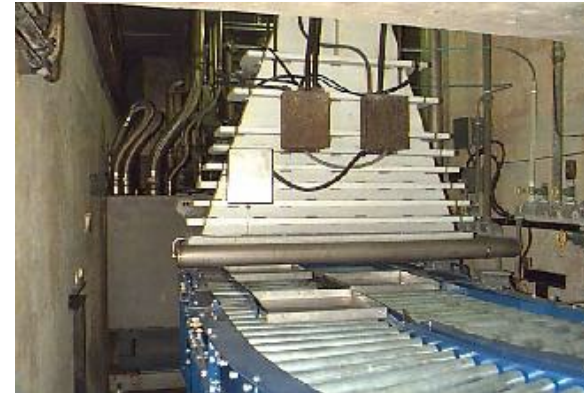
JOB 188 – 1,5 MeV 37.5kW Radiation Dynamics, Inc. (RDI) R&D
