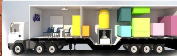
JOB 307 - 97.5 kW, 1.5MeV Continuous treatment system (300 m/min) Commercial applications
