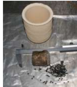
Figure 1 – Uranium ingot, Molybdenum cylinders and Zirconia crucible.
