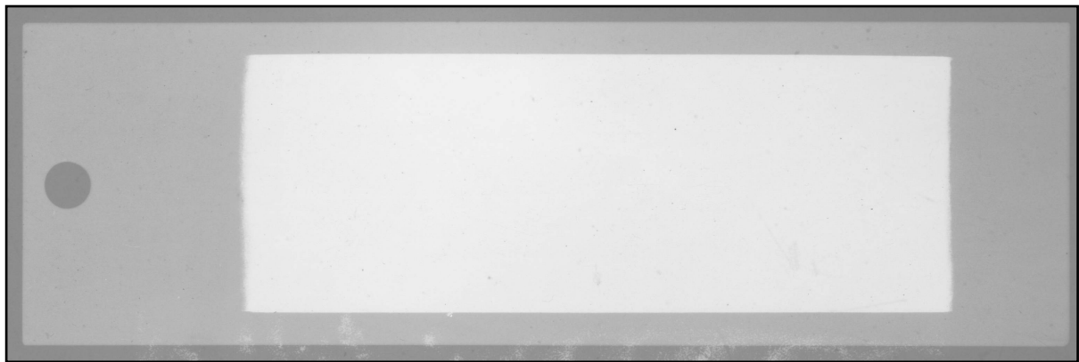
Figure 8. X-ray radiograph taken from U_3Si_2 -Al fuel meat ( 4.8 \text{ gU/cm}^3 ).
