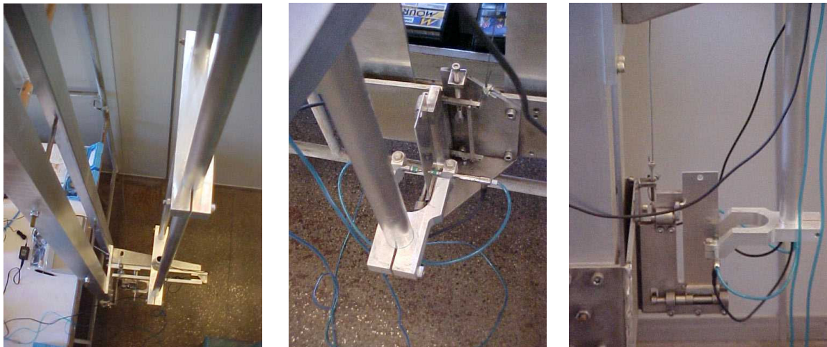
Figure 11. Thickness measurement device: support and miniplate measurement system.
