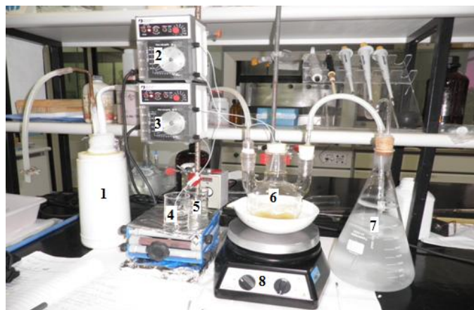
Figure 2. Experimental apparatus used in degradation experiments for a mixture of cationic and anionic resins. 1. Liquid nitrogen. 2 and 3. Peristaltic pumps. 4. Solution of hydrogen peroxide 50%. 5. Solution of catalyst. 6. Resin (anionic + cationic). 7. Solution of calcium hydroxide. 8. Magnetic stirrer (Model 753A, Fisatom).
