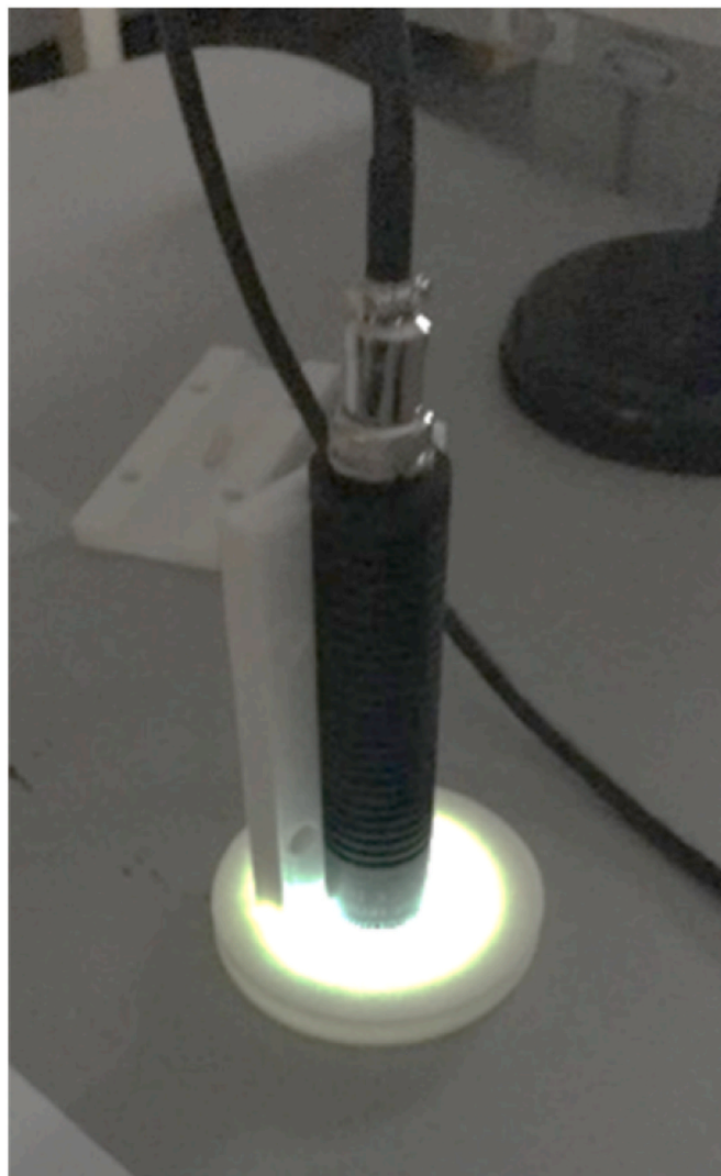
Fig. 1. LED Saber device during an experimental procedure, with illumination of dosimeters.
