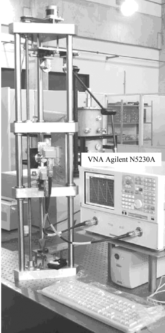
Figure 3. Picture of our home-made setup for measuring dispersion and interaction impedance characteristics of SWS.
