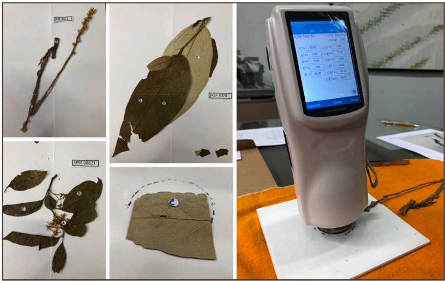
Fig. 2. Identification of colorimetric points and PCE colorimeter measurement set-up.
