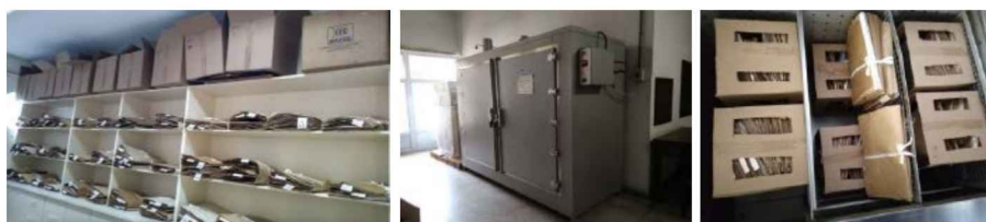
FIG. 23.5. Samples drying naturally and in an oven before processing in the irradiator.
