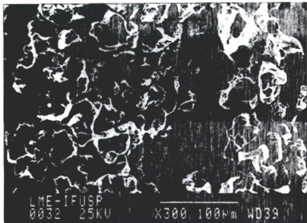
FIGURE 11. As-corroded surface morphology of Steel 347(2) sensitized 13 h at 790°C, after 30 min of immersion in Practice B testing solution. Corrosion was primarily intergranular (SEM, 300x).
