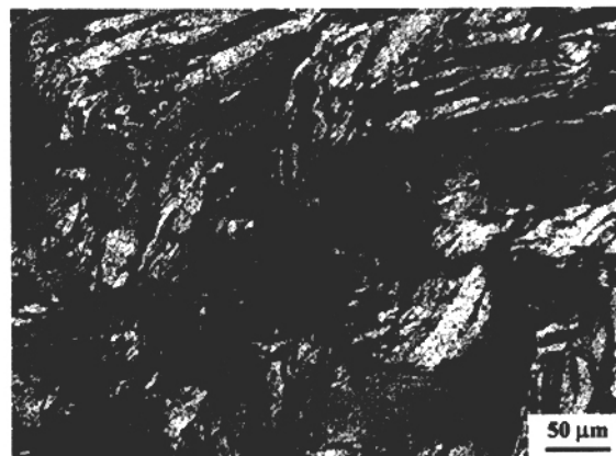
Fig. 8. Transverse section of sample deformed to 72% reduction showing the curly grain structure (LOM).
