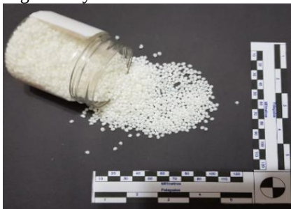
Fig. 3. Polymeric blend of PBAT/PLA
