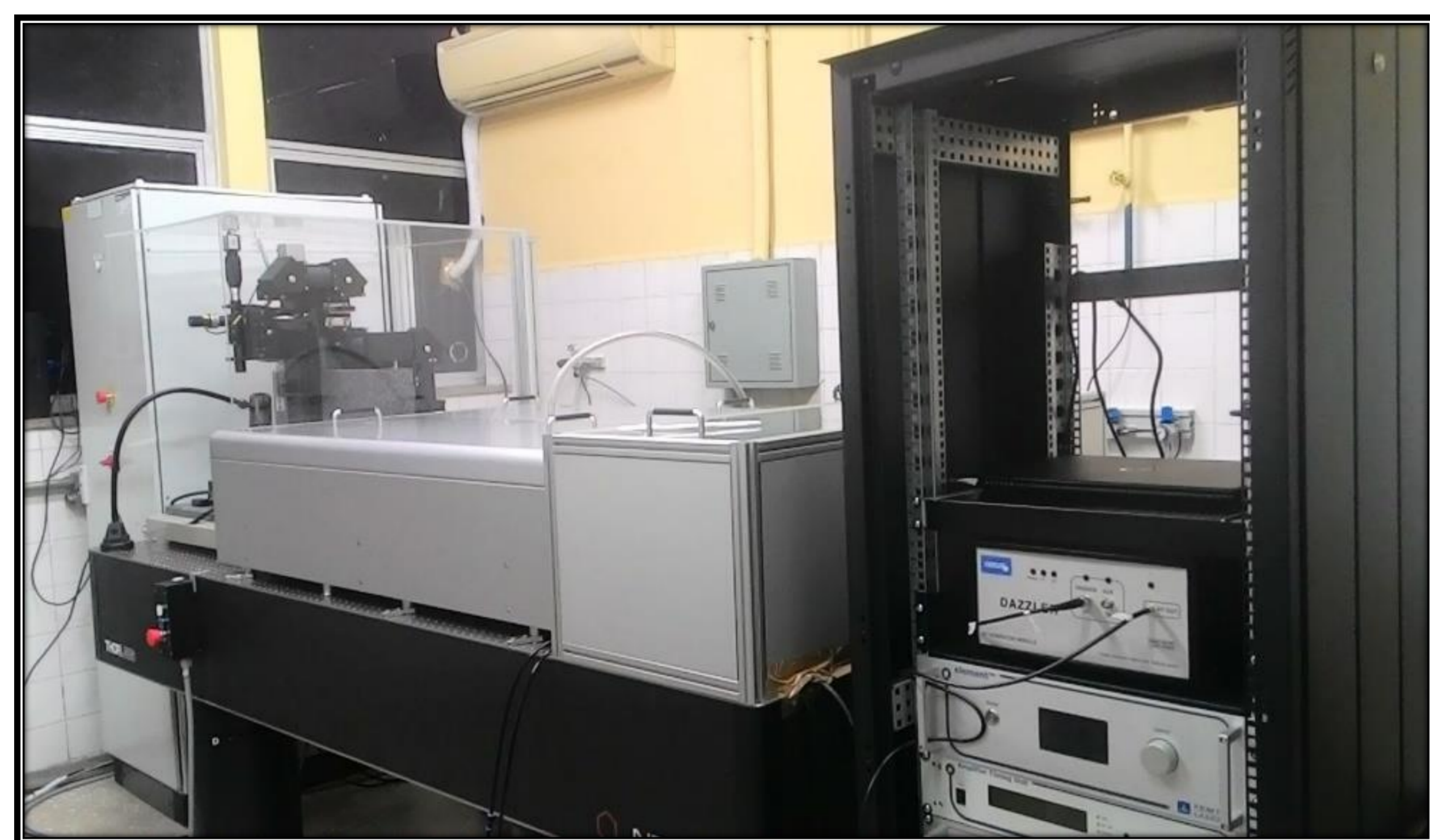
New Femtosecond laser workstation applied in the process of microreactor fabrication
