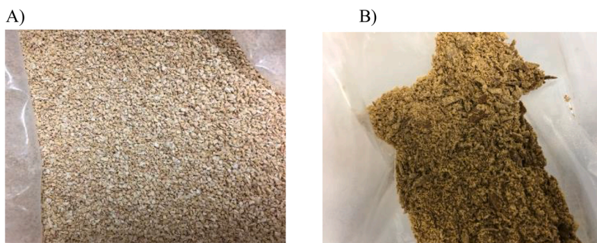
Fig. 1. A) In natura corncob (CC) and B) Extruded corncob with additives (water and glycerol) (ECC-25 %).
