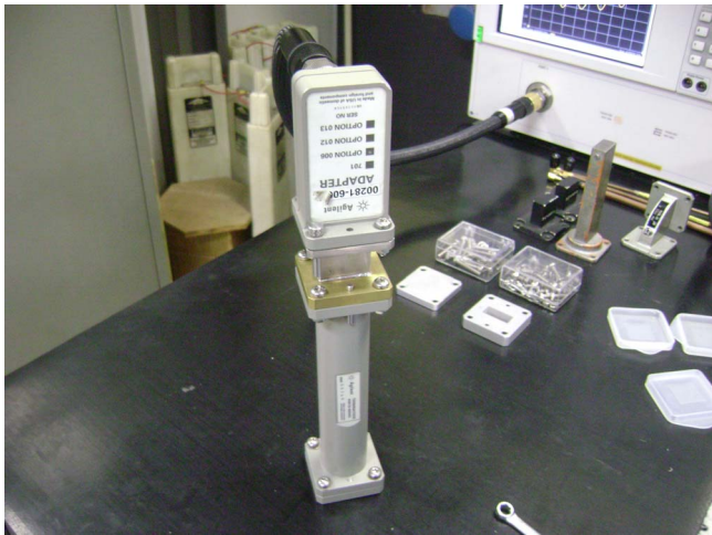
Figure 5 – Experimental set-up used to measure the microwave window impedance mismatching level.
