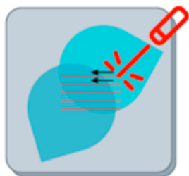
Figure 2. Diagram showing the sample deposition and the overlapping region of ATB (dark blue) and NPs (light blue) as well as the equipment scanning direction (indicated by the black arrows).
