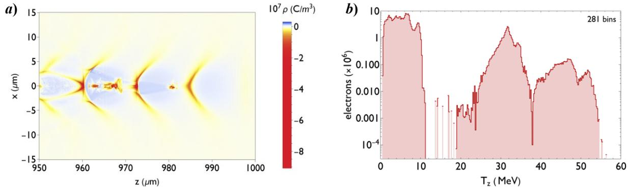
Fig. 1. Results from variation #1: (a) wakefield and entrapped electrons; (b) accelerated beam spectra.
