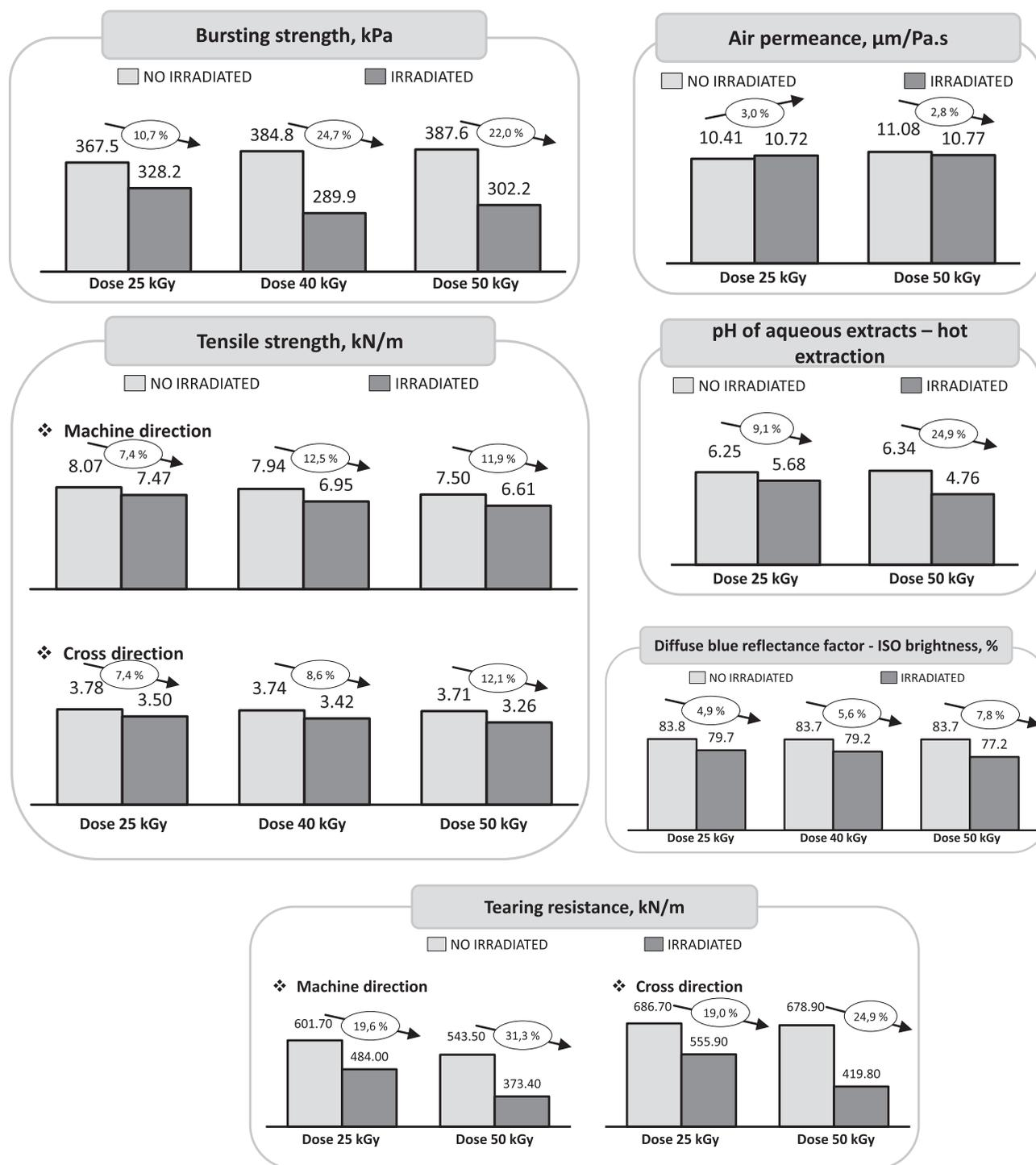
Fig. 3. Radiation effects obtained for bursting strength, tensile strength, tearing resistance, brightness and pH.
