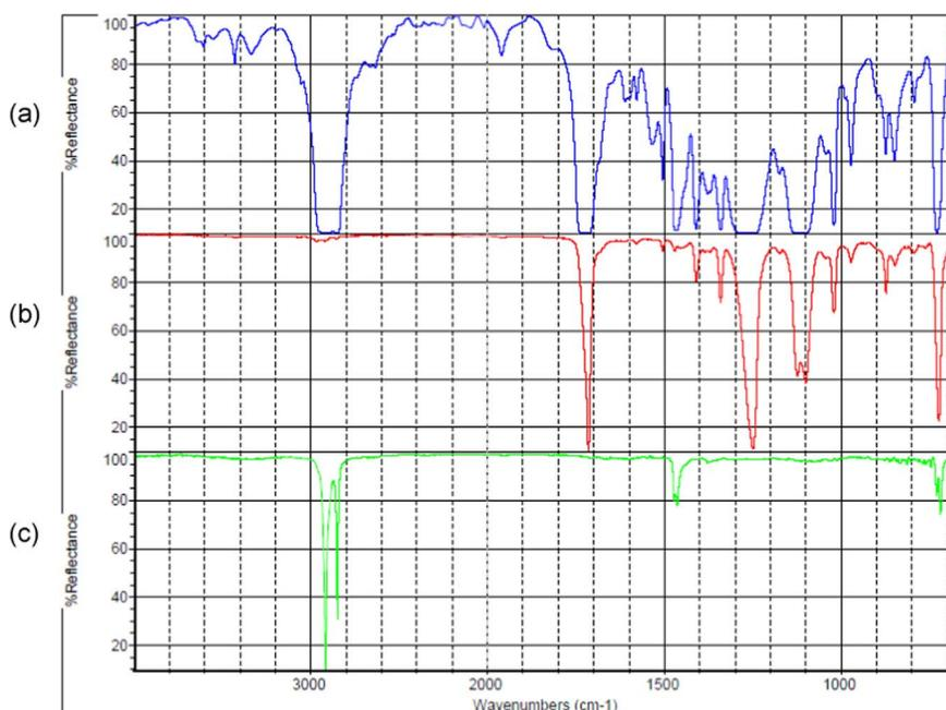
Fig. 2. Infrared spectra of plastic film (a) “full”, (b) “front” and (c) “back”.
