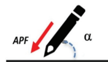
Fig. 1 The axial pen force (APF) related to the position of the pen. The normal force is related to the axial force by F_N = -F_A \sin \alpha .
