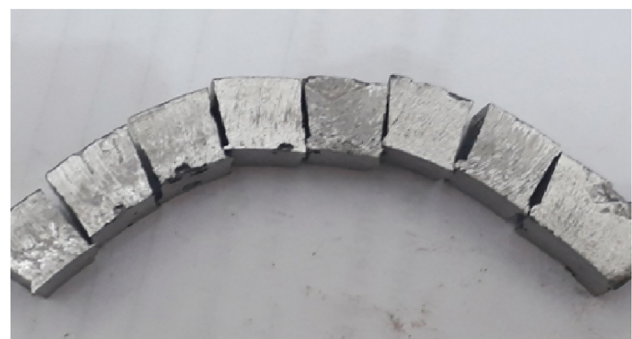
Fig. 4 – Part of the tube ring produced by centrifugal casting divided into 10 samples for micro-abrasive wear tests by a fixed rotating sphere.
