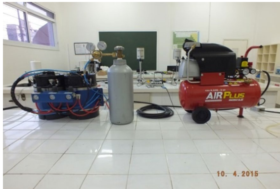
Figure 2. Complete application system of the aqueous-based adhesive, catalyzed by CO 2 . Source: Author's equipment.
